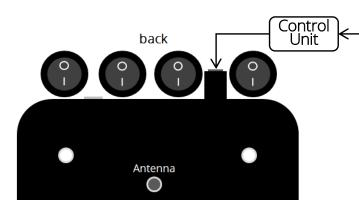
Screw in the antenna; it has to stay in upright position for proper functioning.
