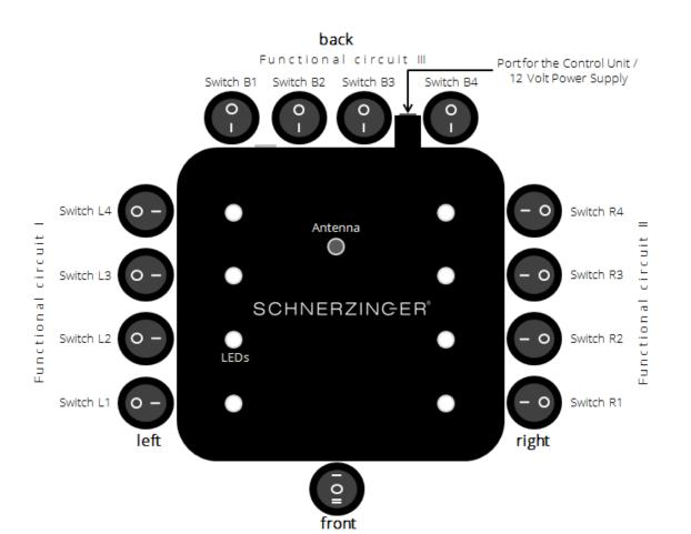
First set the switches of one device in full, then the second device.
